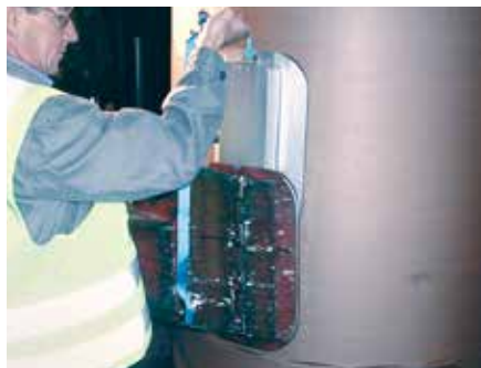
Due to its thin design, the Test Pad adapts to changing roll diameters.
