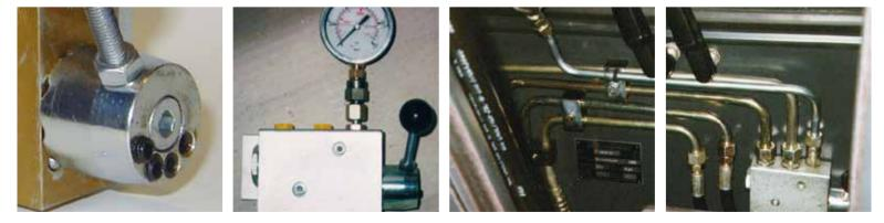
Optional pressure gauge enables easy clamping force monitoring.
