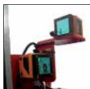
1 Laser detector Laser sensor for upper row to detect presence of boxes in the upper part of the pads.
