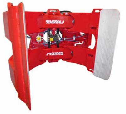
The new Bolzoni Auramo swing frame paper roll clamp range has been designed and developed starting from our long experience on rotating paper roll clamps. The swing movement grants an effective and optimized roll handling also in confined spaces. The swing frame function is able to produce a smooth movement +- 5-degrees left and right, in order to give exact position to the paper roll.
