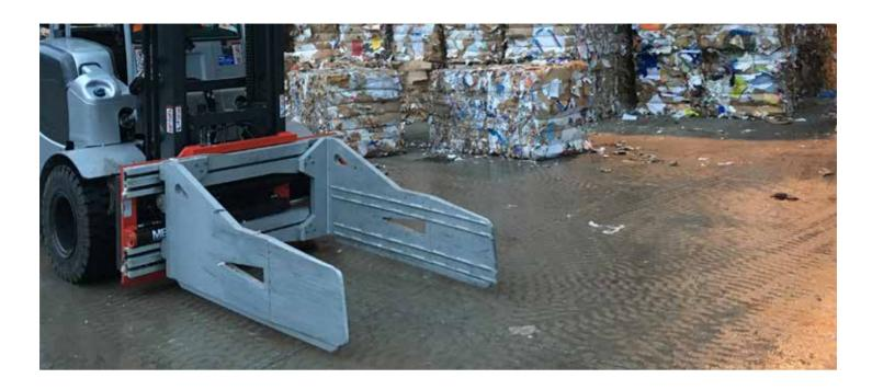
The Bolzoni Auramo series B-400W waste paper bale clamps are designed for heavy-duty waste paper bale handling.
