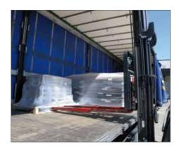
Trucks and trains can be loaded and unloaded from one side: reduction in turnaround space with increase of storage space, saving in time, saving in fuel/battery consumption, manoeuvring reduction with safety improvement.
