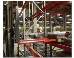
**Double-deep stacking:** increase of storage volumes and remarkable space saving, particularly when combining the Bolzoni Auramo Reach Forks with a reach truck able to work in narrow aisles.
