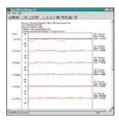
Once the stored data has been downloaded into a standard PC for further analysis and printing, a graphic representation of the surface profile is displayed at each measurement level, with calculated values of maximum out-of-roundness deviations.
