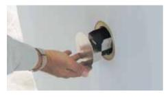
The advanced microelectronics provides a possibility to track the orientation of the paper roll. As the orientation changes, due to roll handling, the Spy will record the change and the time of occurrence and store it into the memory.
