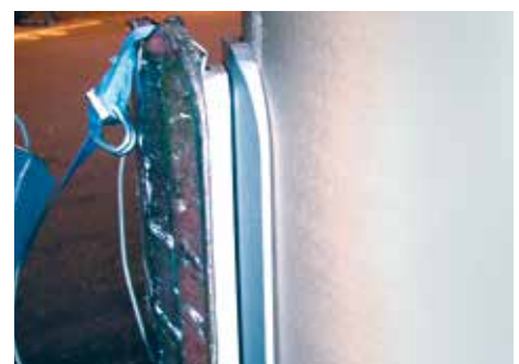
The Test Pad measures the clamping force between the paper roll and the clamp pad.
