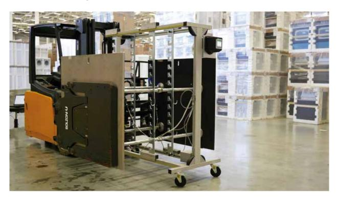
With carton clamps the correct equalization of the clamping force over the surface of the pads is a KEY factor to ensure the most appropriate handling of white and brown goods. All Bolzoni carton clamps are tested at the end of the production line with the 4-Point Dynamometer specifically designed by our research & development center to grant the correct factory set up of the clamp and allow proper recalibration of the force distribution after a certain period of use.
