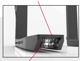
High quality camera with LED lights completely integrated in the fork tip
