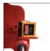
③ Depth load engagement sensors Detect type and configuration of the load in depth/height and the distance from the clamp body.
