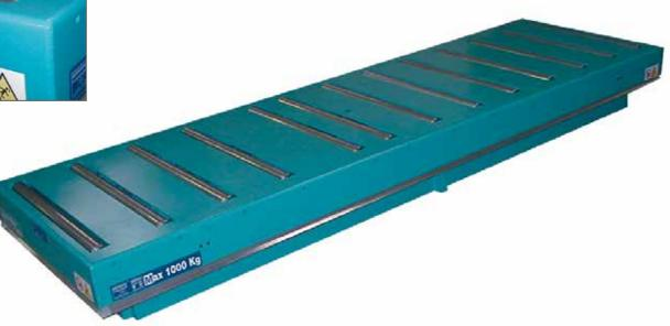
The lift table with integrated conveyor is mainly used in the wood working industry, to handle furniture, doors and paneling, in particular on the pressing lines.
