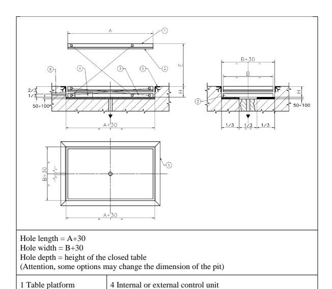
5 Pit edge protective angle bar (L profile 60x60 mm)
