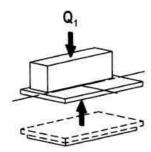
33% of the rated load (maximum load) distributed evenly over half the table width.
