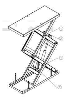
1-Central pivot 2-Cylinder coupling pin (Elevated cycles)
